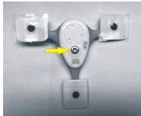
**Figure 14. QuoreOne with the electrodes fitted. The arrow indicates the central electrode.**
