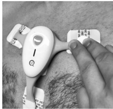
**Figure 18. Pressuring the electrode to ensure good quality of adhesion.**
