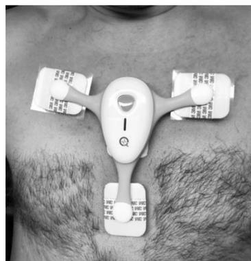
**Figure 16. QuoreOne with the central electrode connected to the electrode on the body.**
