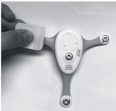
**Figure 13. Fitting the electrode to QuoreOne.**
