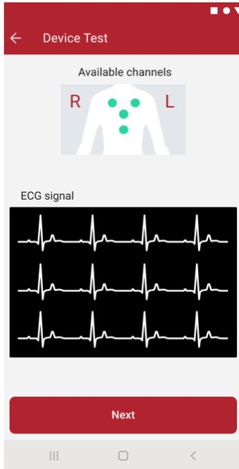
Figure 31. Visualization of signal and status of the electrodes.
